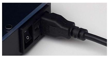
The 24 V DC voltage supply is fused with 1.6 A.
