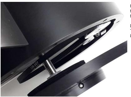
For renewed installation carefully lift the wheel on the axle with both hands. Gently push the drive belt onto the drive wheel with your fingertips by moving back and forth.
