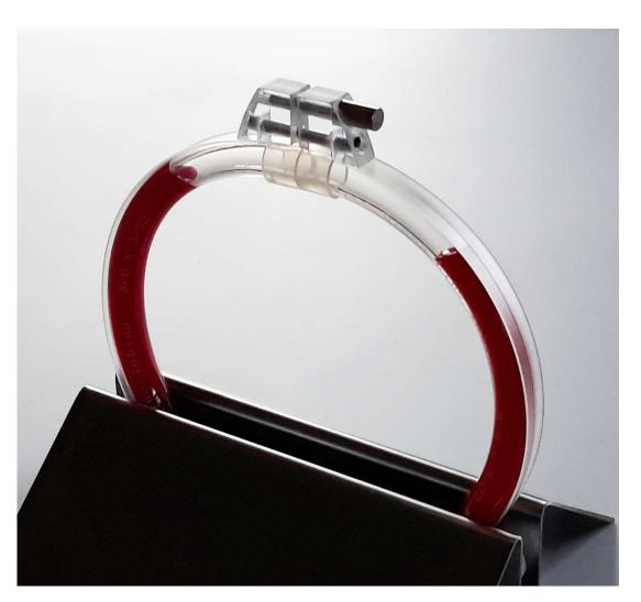
The tube connector is a technological development of the conventional connection of tubes with a short piece of bigger sized tubing. An additional polycarbonate tension band around the loop leads to perfect fit and sealing at the splice. Its length can be varied and adjusted. A regulation of the closing force at the sealing surfaces is implemented.
