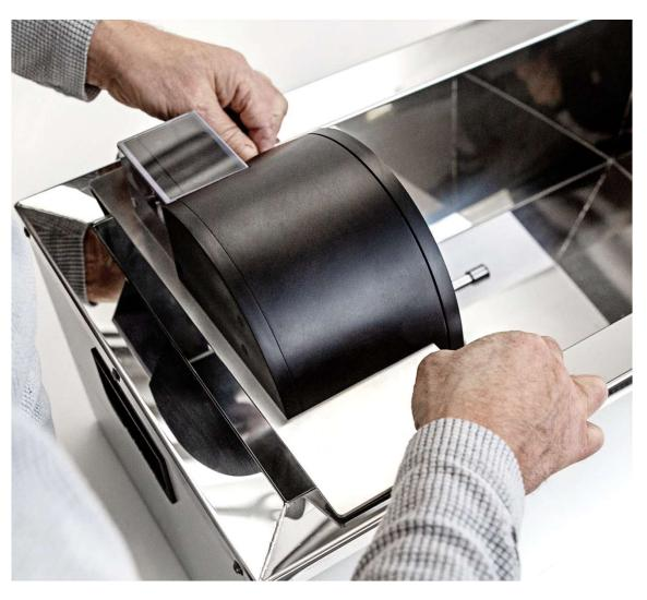
The drive is inserted into the water bath from above. Fastening is not necessary
