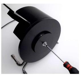
After loosening the center screw, the drive wheel can be taken off for inspection
