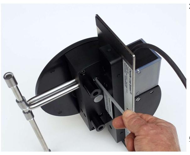
On the underside, there are adjustable metal brackets as stands. Their position can be fixed with the associated screws.
