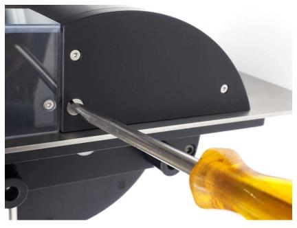
A small clockwise turn increases the belt tension
