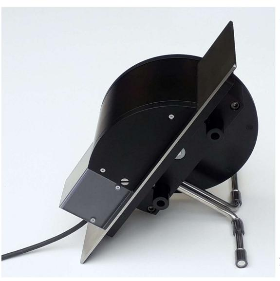
For incubator setup, please arrange the brackets as shown. Alternatively, the rotation unit can be also placed mirror-inverted at the left side of the loop cradle, using the other pair of mounting holes. In this case, the cable entry is from above.
