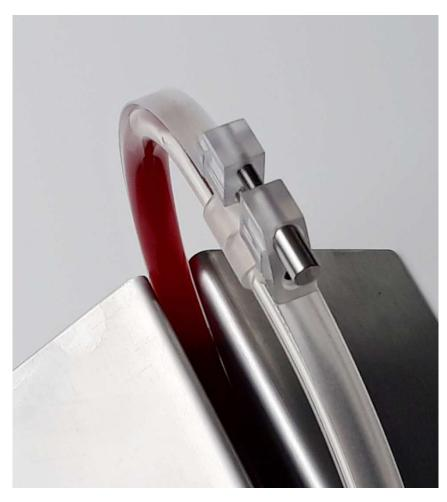
press the loop inside the tension ring
